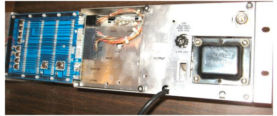
The new "rear" access contains the back-plane board for external connections and the RF port.
